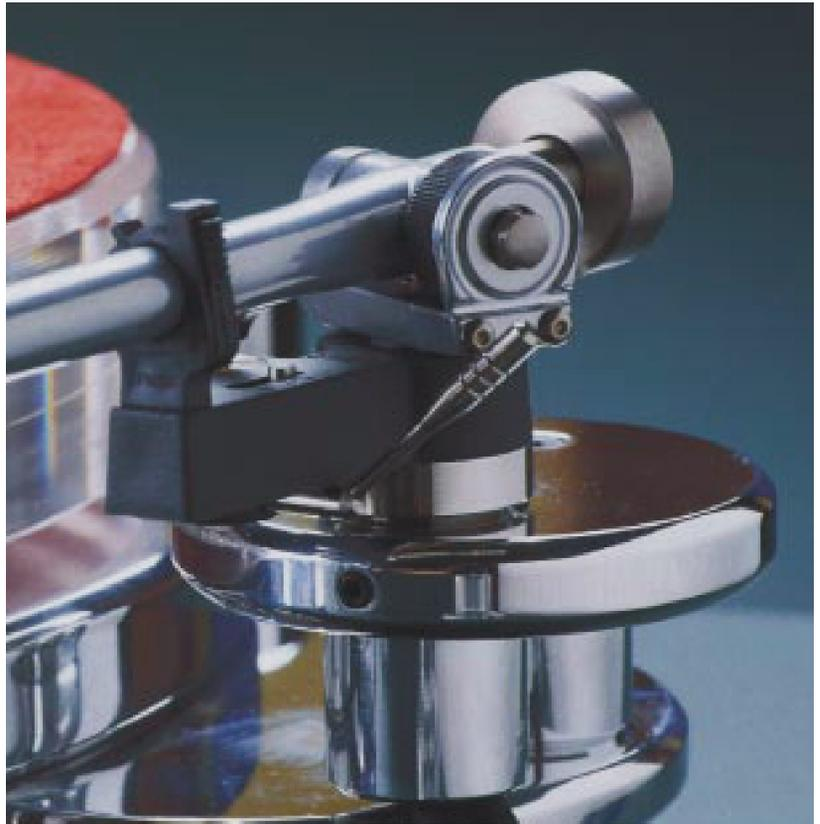
controls the arm's freedom of movement. The main counterweight is off-center to enable horizontal balancing. With a small supplementary weight the bearing load can be adjusted. The head shell and
