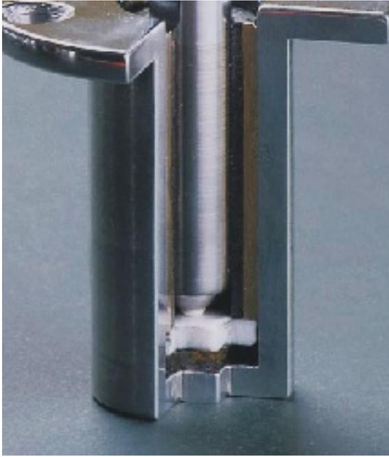
**A ceramic ball moves on a Teflon plate: the Solid Machine's bearing clothed in plastic.**
